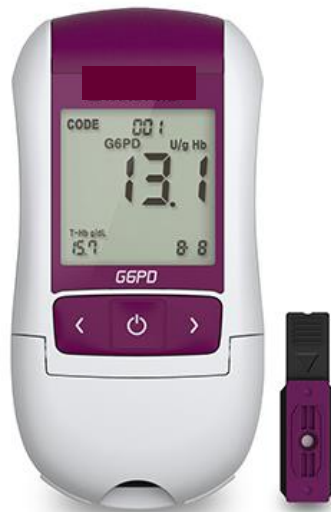
Figure 4 Quantitative G6PD test. The analyzer displays G6PD enzyme level in U/gHb on the screen
